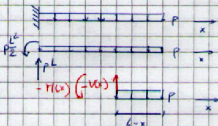
$$\begin{aligned} -V(x) - p(L-x) &= 0 \quad \text{donc} \quad V(x) = -p(L-x) \\ -M(x) - p \frac{(L-x)^2}{2} &= 0 \quad \text{donc} \quad M(x) = -p \frac{(L-x)^2}{2} \end{aligned}$$
